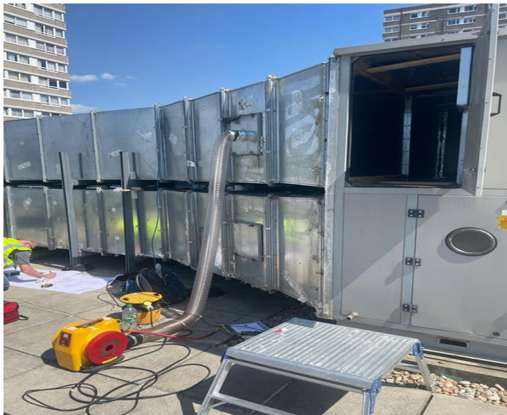
Installation of the Retrotec 451 tightness tester attached to the ductwork before testing took place.
