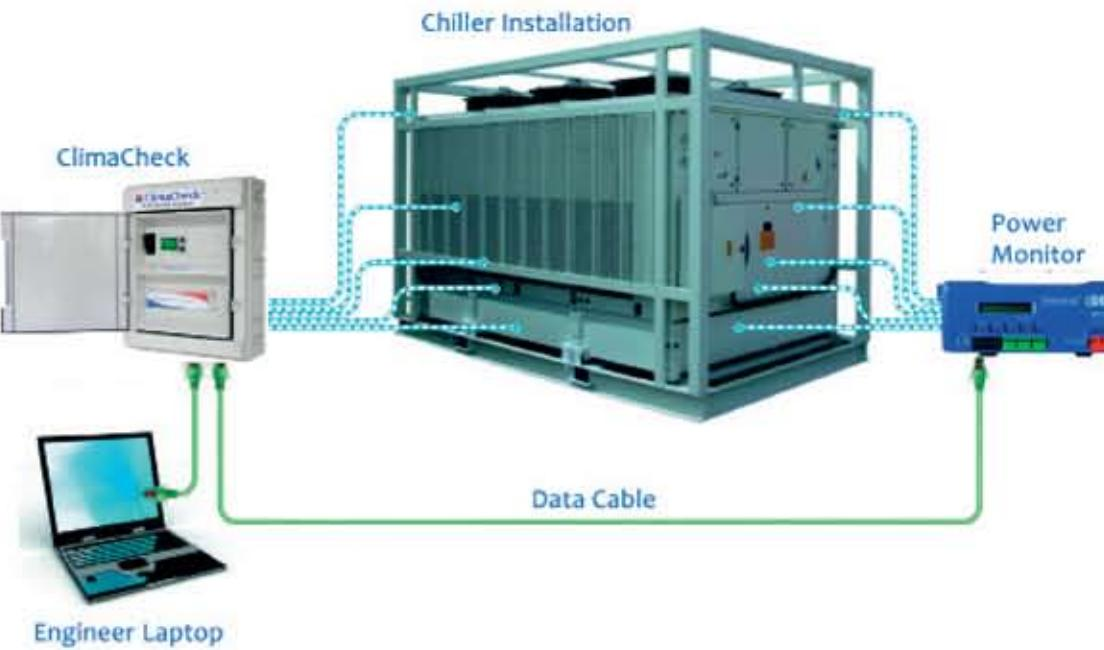
power consumption, cooling performance, thermal load of the system, as well as chilled water temperatures and flow rates along with refrigerant conditions such as sub-cooling at the expansion valve inlet and superheat at the compressor inlet. ClimaCheck is unique in providing this data based on the power consumption of the compressor as well as the refrigerant thermodynamic cycle as measured on site, without the need for refrigerant or water flow meters.
